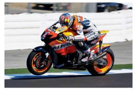
NICKY HAYDEN'S TOP SPEED, reached at the Chinese Grand Prix in May. MotoGP bikes, which weigh about 300 pounds and produce more than 220 horsepower, are among the fastest accelerating machines on earth (0 to 62 in 2.1 seconds); at full throttle, their engines rev at more than 18,000 r.p.m.'s.
